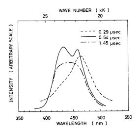
Figure 1. The time-resolved spectra of polycrystalline  ${\rm K_2Pt}\left({\rm CN}\right)_4.3{\rm H_2O}$  .
