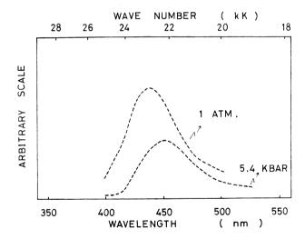
Figure 2. The pressure effect on the luminescence spectra of polycrystalline  ${\rm K_2^{Pt}(CN)_4.3H_2O}$ .
